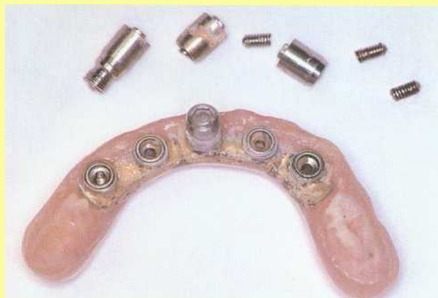
Fig 3-18 Loosened prosthesis. The placement of the implants in-line, in combination with the large extensions, leads to a risk of mechanical complications, especially if this situation is combined with an unfavorable occlusal context. After several incidences of screw loosening, the abutment screws and two implants fractured.
